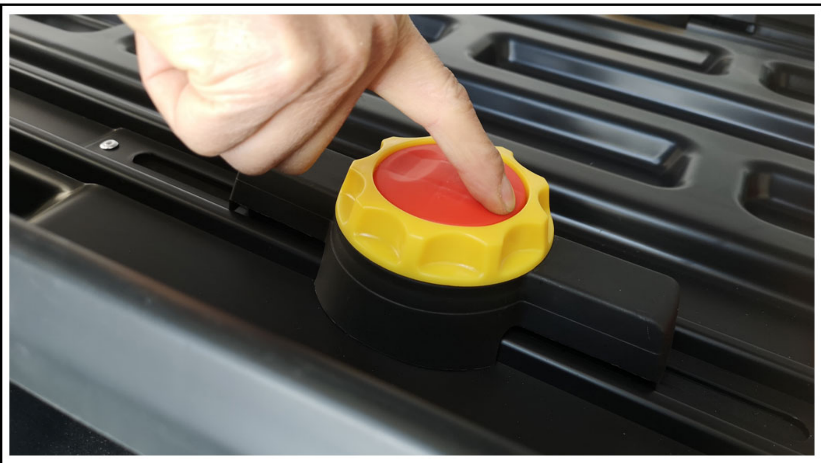
11. Press the other end of the quick clip to close.
