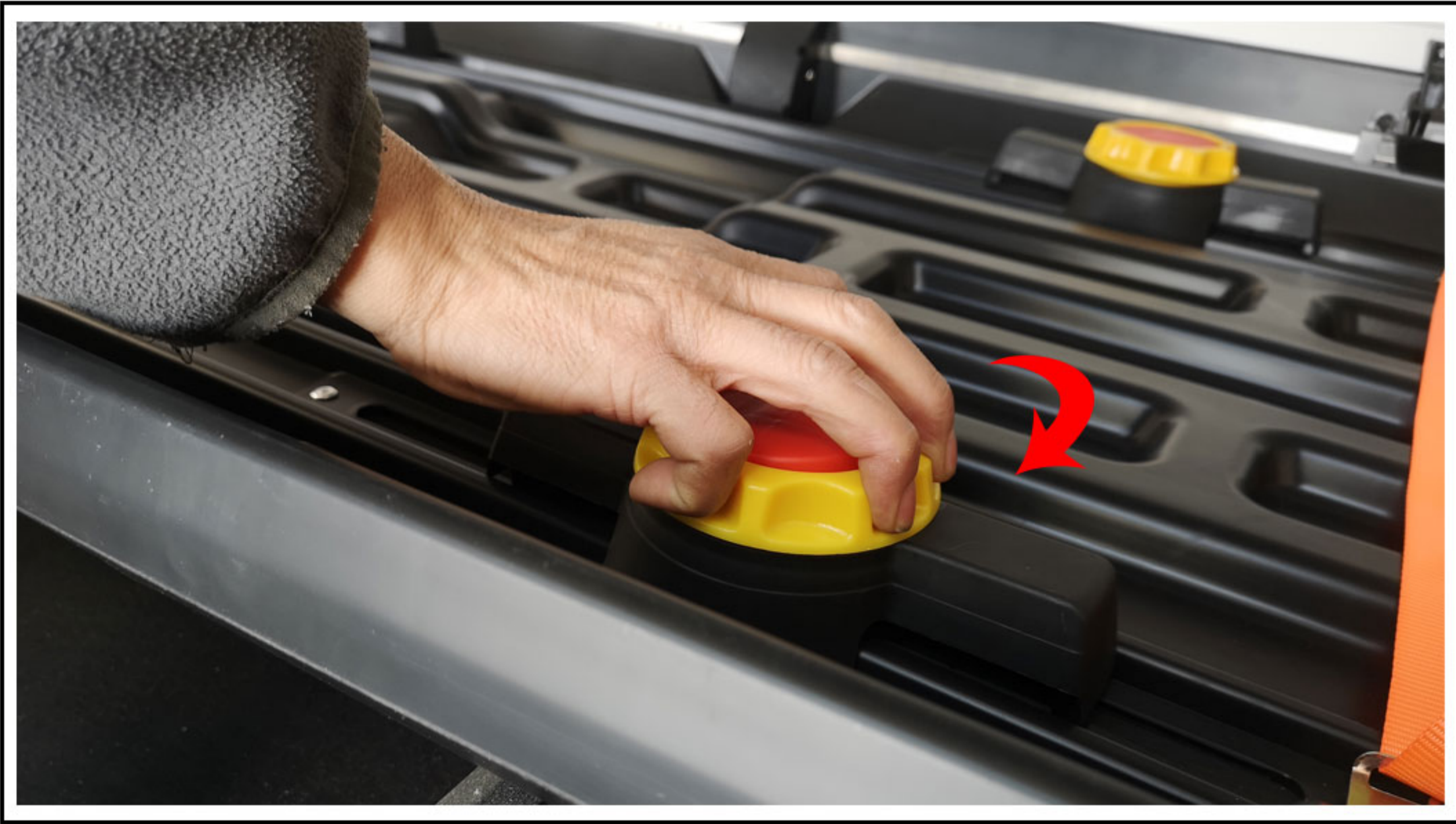
9. Turn the quick clips clockwise to lock.
