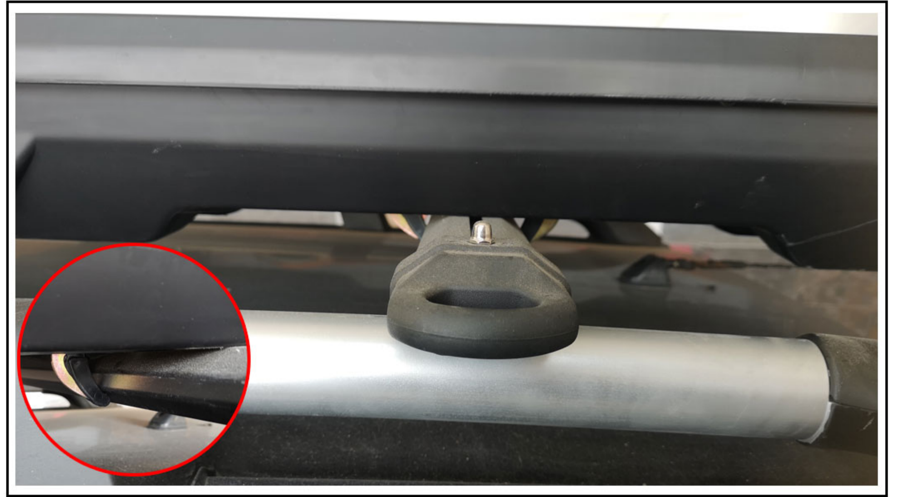
10. Quick clips lock cross bar.
