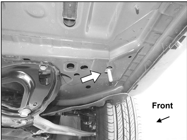
(Fig 14) Insert "Long" Bolt Plate into oval hole in front floor location (arrow)
