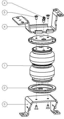
Figure 1: Air Spring Pre assembly
