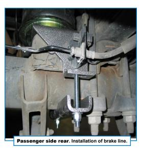
Using the M8 cap screws, attach the emergency brake cable bracket to the lower bracket of the air bag assembly on the passenger side of the vehicle.
