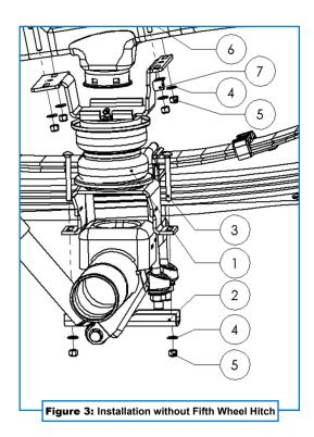
15 Secure the emergency brake cable on the driver side of the vehicle with the adel clamp (7). Mount the adel clamp on the U-bolt, under the air bag bracket, forward of the jounce bumper on the inside of the frame.
