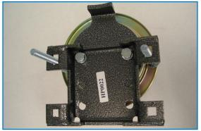
The lower bracket is designed to be installed offset to the lower end of the air spring. The offset must be opposite the air fitting installed in Step 4.
