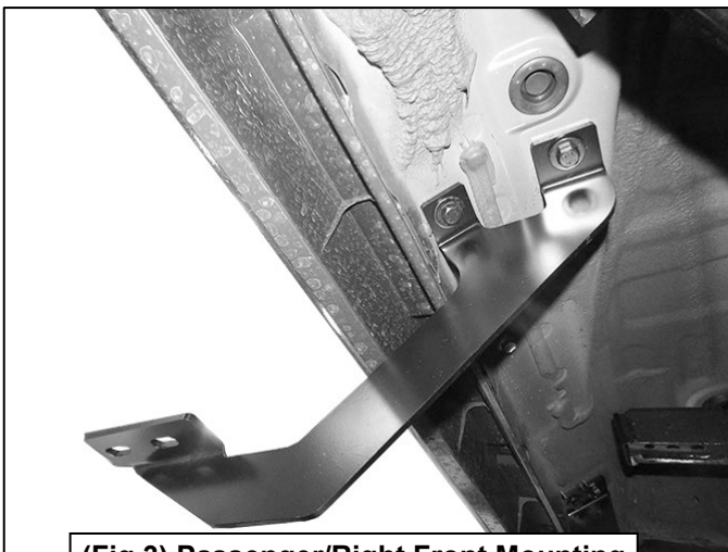
(Fig 3) Passenger/Right Front Mounting Bracket attached to the front location
