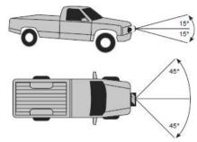
16. If the object to be pulled must be pulled at an angle in relation to the winch, use a pulley (sold separately) and an anchor point directly in front of the winch, as shown in the following picture.
