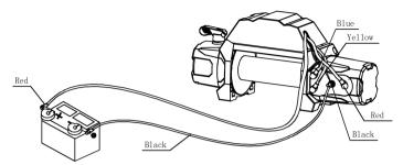
4. Attach the red, black and blue cables to their corresponding terminals on the winch.
