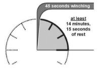
continuous operation. Failure to carefully observe duty cycle limitations can easily overstress a winch, causing premature winch failure. Do not attempt to pull full rated load for more than 20 seconds. Release Power-In switch immediately when winch drum/rope stops. Allow winch to cool and change rigging as needed before continuing pull.
