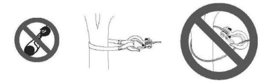
Do not wrap the rope around the object and hook onto the rope itself. This can damage the object being pulled, and kink or fray the rope.
