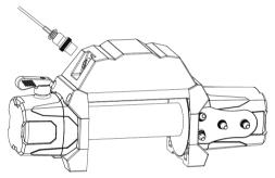
13. Operate the wired remote controller briefly to ensure the controls work properly. If operation is reversed, the power cables may be connected backwards. Correct any such issue before use.
