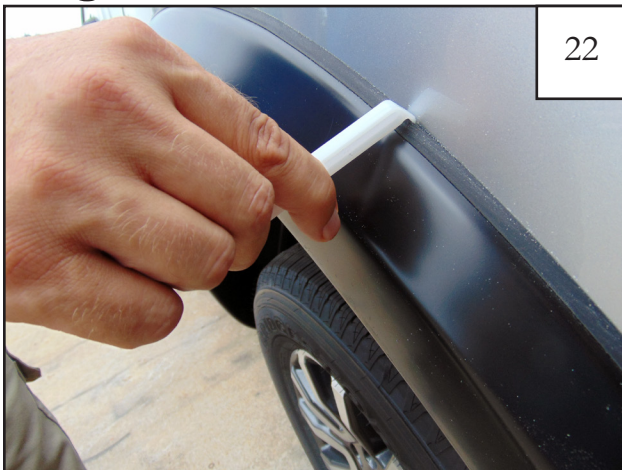
Using supplied Edge Trim Tool (Item 11), seat edge trim against vehicle by hooking curved end under edge trim at one end of flare. Next, slide around outer edge of flare to the other end.
