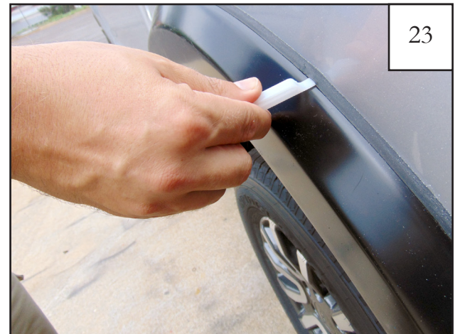
Using flat end of supplied Edge Trim Tool (Item 11), seat edge trim against flare by inserting straight end between edge trim and flare at one end. Next, slide around entire edge to the other end.
